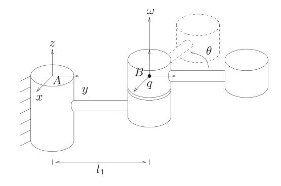
• What is the screw axis for twist  $\mathcal{V} = (0, 2, 2, 4, 0, 0)$ ?
